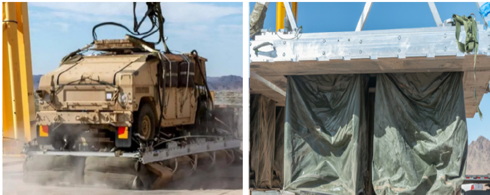
图 6 RRDAS 空投系统缓冲气囊 Fig.6 Rapid Rigging De-Rigging Airdrop System cushioning airbags
