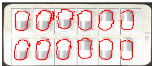
图 16 未补光目标结合 HSV 识别结果 Fig.16 Recognition results of target combined with HSV under no supplementary light
