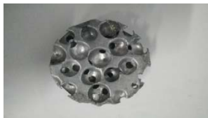
图 1 泡沫铝试样 Fig.1 Aluminum foam sample
