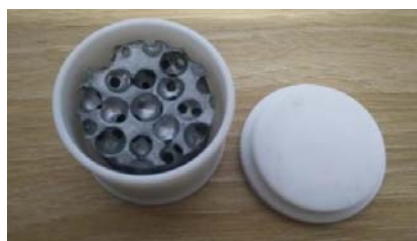
图 2 放有泡沫铝的模具 Fig.2 Mold with aluminum foam
