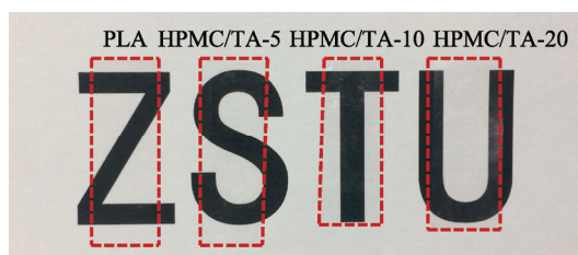
图6 PLA原膜及不同组装层数PLA薄膜的透明性 Fig.6 Transparency of original PLA film and PLA film with different number of assembly layers
