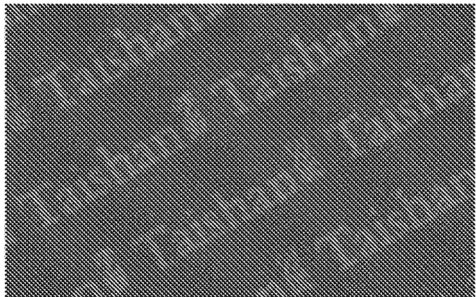
图 4 光栅片线条角度与印刷品呈 135°时效果 Fig. 4 Effect of grating line screen angle on printing at 135°
